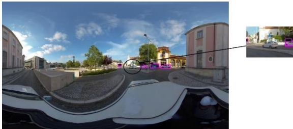
Figure 1: Predictions in ERP images. DL algorithms show more difficulty detecting objects in centre regions.
