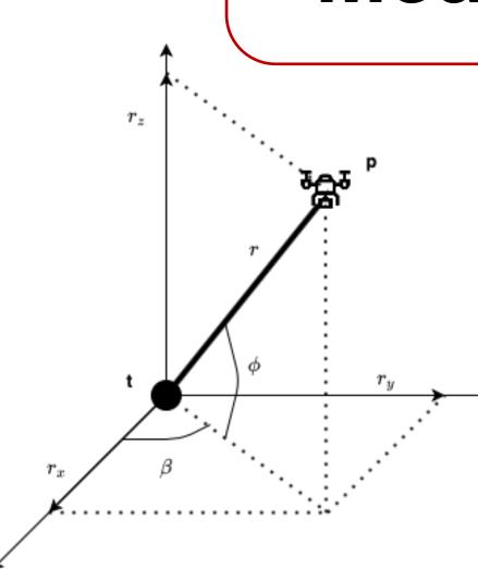
A new **Bearings-Range** measurement model was developed to filter multiple IRT estimates of the same stationary target.
